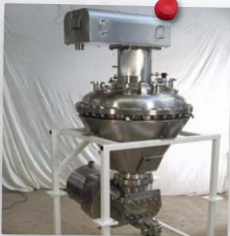
SSIP agitated screw feeder 2003
