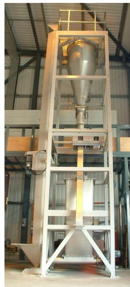
*The Ajax static screw elevator will transfer material in a more densified and settled condition than a conventional screw elevator.*
