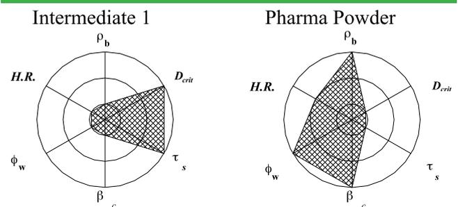
This technique when applied to two other examples highlights particular aspects of the 'profile' that merit special attention. Intermediate 1 shows the resultant diagram for a chemical intermediate 1; all aspects for flow are good except the shear strength and outlet size. To overcome potential flow problems for batch handling of this material invertible IBC bins were used with a larger outlet that upsets the consolidation of the material to ensure reliable flow to process.
