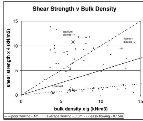
Figure 3: Data from shear tests plotted in sectors partitioned by constant outlet size to indicate easy modest and poor flow characteristics.
