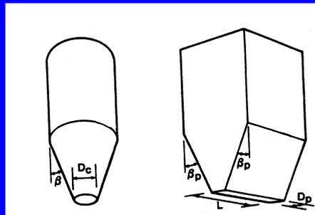
*Getting the right hopper shape for flow. Mass flow wall angles are predicted from wall friction tests but plane flow shapes can have shallower walls than cones*
