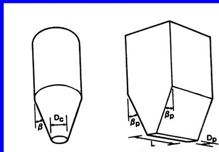
*Getting the right hopper shape for flow. Mass flow wall angles are predicted from wall friction tests but plane flow shapes can have shallower walls than cones*
