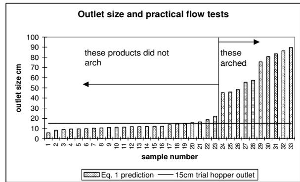
Fig. 2: Predicted outlet size compared with flow behaviour in hopper.
