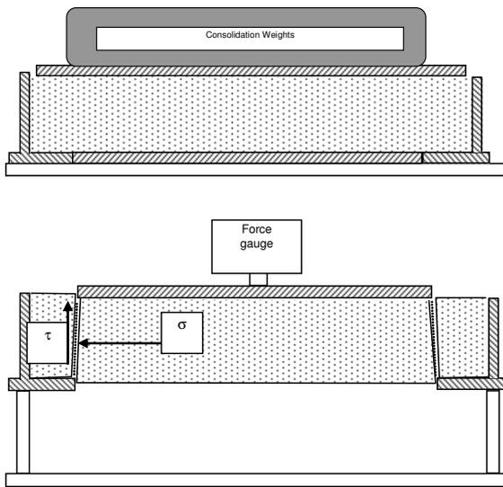
Figure 1 Vertical Shear Cell test: stage 1 – consolidation; stage 2 – shearing stage.
