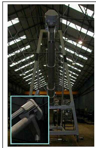
In a design innovation, the elevator drive motor is mounted half way along the screw length for better balance and ease of maintenance.
