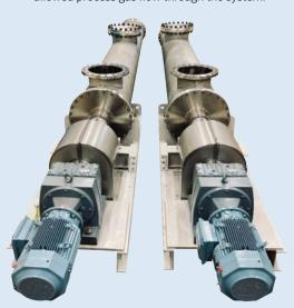
Whilst wall friction affects the efficiency of axial transfer and is an important aspect for selecting a suitable transfer pitch, particularly when the conveyor needs to be inclined, some poor flow materials, such as damp salt, soon expose any 'standard screw' deficiencies, in some cases causing blockages which damage the machine and interrupt production.
