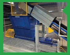
When Binding Solutions Limited (BSL) was developing a plant for its technology to improve steel making, Ajax Equipment was selected to supply a feed system for a mix of iron ore and additives. Ajax's scope comprised buffer hopper, screw feeder and agitated screw feeder.
