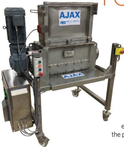
Vickers Laboratories has enhanced production with a combined mobile lump breaker and sack-tip featuring a pharmaceutical grade, stainless steel finish from Ajax. The system allows sacks of caked pharmaceutical powders to be safely opened and efficiently reduced to a consistent particle size, while the mobile frame enables the station to be removed from the production line and fully washed down.
