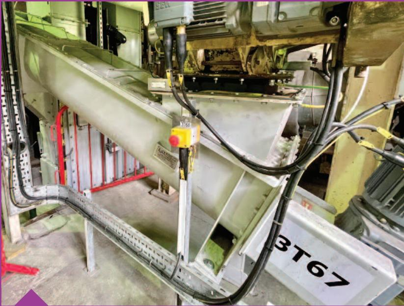
Speciality chemicals and sustainable technologies company, Johnson Matthey, has enhanced the handling of a catalyst material at temperature with an inclined screw conveyor and chute sections from Ajax.
