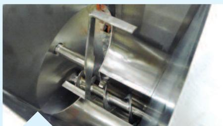
Inside a retractable screw feeder with Z-form agitator.
