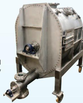
Design wise, mechanical integrity, assessment of the torque required and how that is delivered, e.g. using planetary geared motor units, and matching with the screw for feed control are very important, especially on 'supersized' machines.
