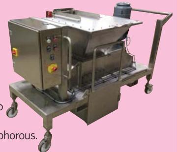
The stainless steel lump breaker features an integrated control panel and a number of operator safety features. These include sliding safety gates to restrict side access to the discharge area during operation, and Rotacam safety switches fitted to the integral holding hopper and hinged cover.
