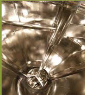
Bulk pharmaceutical compound is tipped from a big bag into the agitated screw feeder's large hopper section allowing gravity flow to a robust, multi-bladed agitator, and screw feeder. The auger features a stepped shaft with variable pitch, to pick up the cohesive powder progressively from the full length of the agitated feeder outlet.
