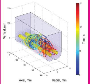
Positron Emission Particle Tracking (PEPT) for the Characterisation of Mixing Properties inside the AJAX Twin Screw Mixer. University of Birmingham, Project Chariot
